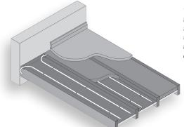
"When mixed floor solutions are being served from the same manifold, a floor probe must be used in the floor solution with the lower maximum supply temperature. This is to limit the temperature in these floor areas and prevent damage to the floor solution and/or floor finish."
